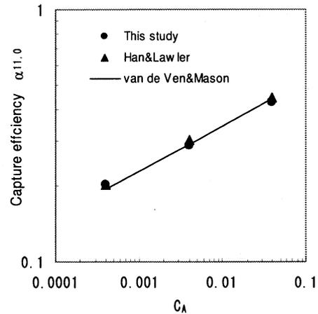
Fig.3 Capture efficiency of homoaggregation without EDL force.
