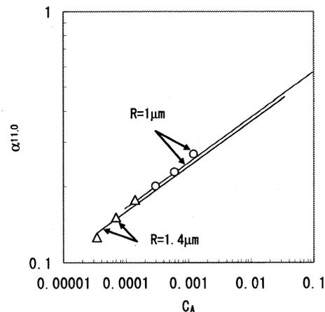
Fig.5 Capture efficiency of homoaggregation ( $R_1=R_2=R$ ) without EDL force. Experiments (symbols) are compared with calculations (Lines). To obtain better fits,  $A_{12}$  ( $10^{-21}$ J) =3 and 1 are assumed for  $R=1$  and  $1.4 \mu\text{m}$ , respectively.
