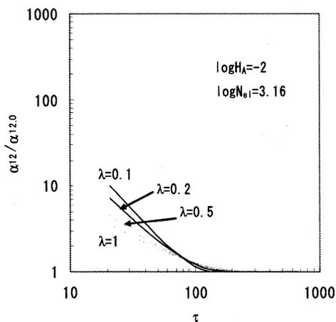
Fig.6 Capture efficiency of heteroaggregation between unequal-sized spheres with attractive EDL force.
