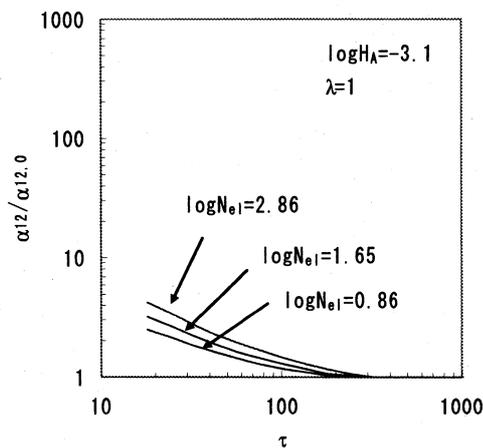
Fig.8 Capture efficiency of heteroaggregation between unequal-sized spheres with attractive EDL force.
