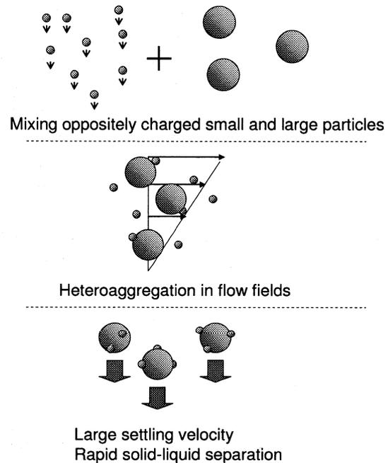
Fig.1 Schematic illustration of heteroaggregation and its application; heteroaggregates enhance solid-liquid separation.
