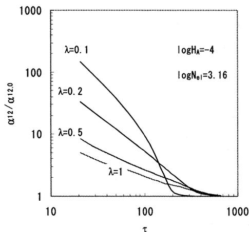
Fig.7 Capture efficiency of heteroaggregation between unequal-sized spheres with attractive EDL force.
