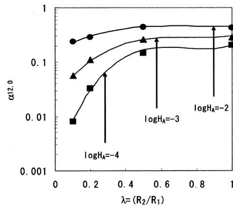
Fig.4 Capture efficiency of heteroaggregation without EDL force: Symbols and lines are evaluated by this work and by Eq. (5), respectively
