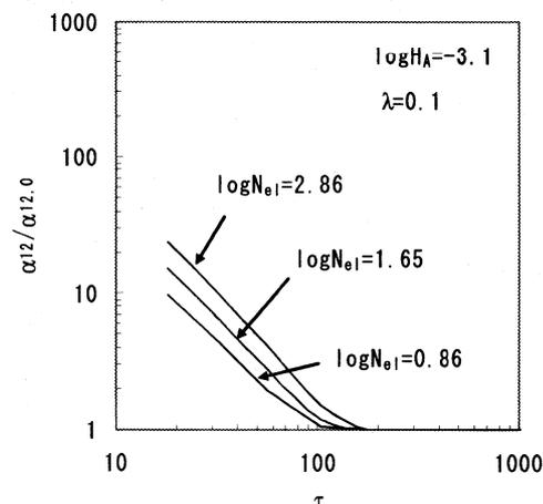
Fig.9 Capture efficiency of heteroaggregation between unequal-sized spheres with attractive EDL force.
