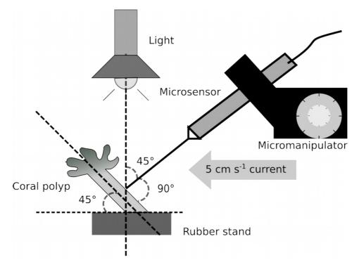
Figure 1 Schema showing the set-up used for microsensor measurements. Individual coral polyps were fixed on rubber stands and placed in a custom flume under a 5 cm s<sup>-1</sup> current. Light at 200  $\mu$ mol s<sup>-1</sup> m<sup>-2</sup> was provided by a metal halide lamp.
