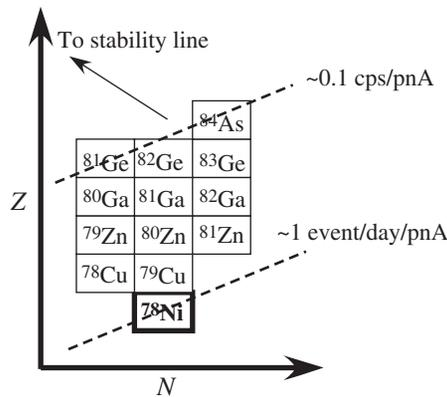
**Fig. 6.** Nuclear chart related to the  $^{78}\text{Ni}$  mass measurement. The nuclei to be injected into the rare-RI ring accompanied by the  $^{78}\text{Ni}$  beam are shown. Broken lines show the rate in the rare-RI ring. The calculation was done by using LISE++ [25].
