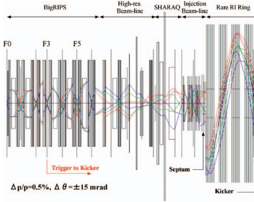
**Fig. 5.** Ion-optical calculation of the injection beam-line (from F0 in BigRIPS to the kicker magnets in the cyclotron-like storage ring). Red, green, and blue lines correspond to particles with  $\delta p/p = +0.5\%$ ,  $0.0\%$ ,  $-0.5\%$ , respectively.
