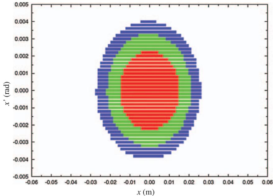
**Fig. 4.** Emittance for a good isochronicity region for  $x$  calculated by our simulation program. The red region shows the area where the isochronicity is  $< 10^{-6}$ . The green and blue regions show the area where the isochronicity is  $< 2 \times 10^{-6}$  and  $< 3 \times 10^{-6}$ , respectively. The results show the isochronicity after 2000 turns in the rare-RI ring.
