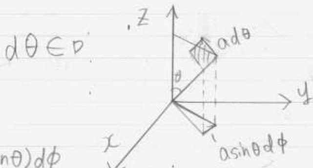
$$ad\theta \times (a \sin\theta) d\phi \\ = a^2 \sin\theta d\theta d\phi$$
