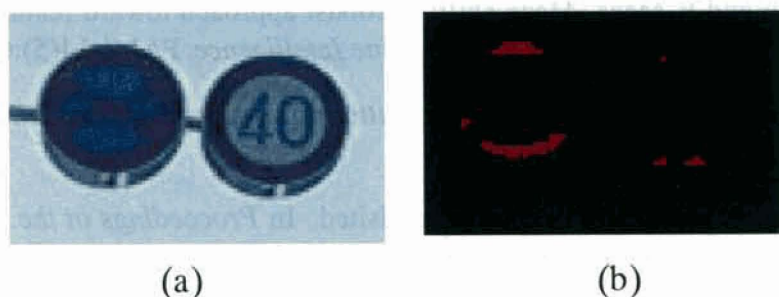
Figure 8: An example of detection failure. When road signs are seen against bright sky as shown in (a), the hue of red annuli black out and they cannot be detected as shown in (b).
