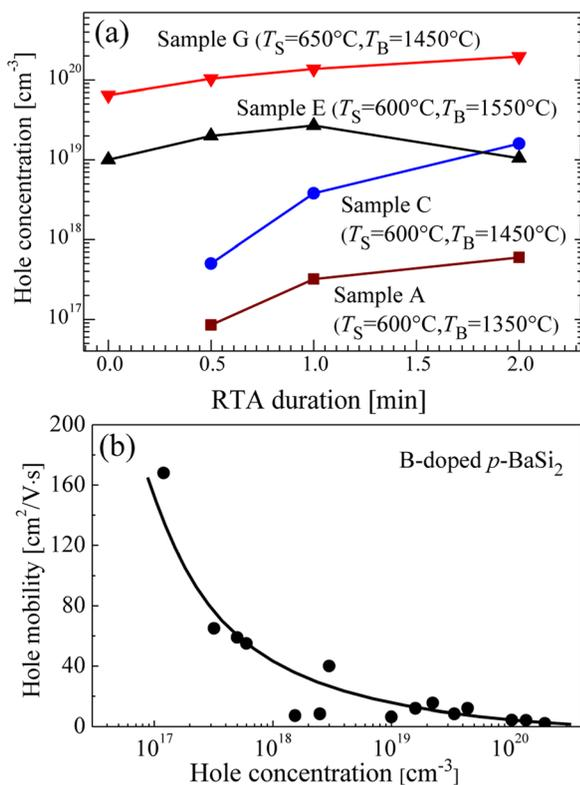
FIG. 3. (a) Dependences of hole concentration on  $t_{\text{RTA}}$  for samples, A, C, E, and G, and (b) relationship of measured mobilities and hole concentrations for B-doped  $p$ -BaSi<sub>2</sub>, grown at  $T_{\text{B}} = 1350$ – $1575$  °C. The solid line is a guide to the eye.
