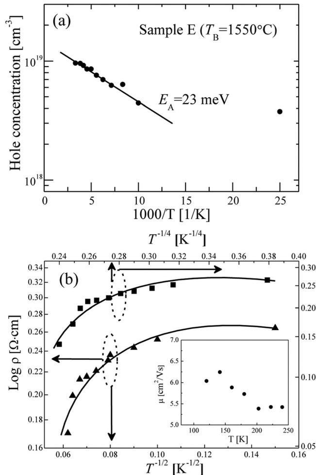
FIG. 2. (a) Temperature dependence of hole concentration and (b) logarithmic dependence of resistivity on  $1/T^{1/2}$  and  $1/T^{1/4}$  for sample E, B-doped *p*-BaSi<sub>2</sub> grown with  $T_B = 1550$  °C. Temperature dependence of mobility for sample E was inserted.
