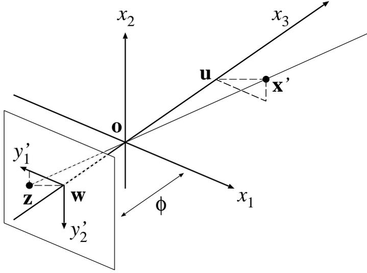
Figure 1: Geometry of a pinhole camera.
