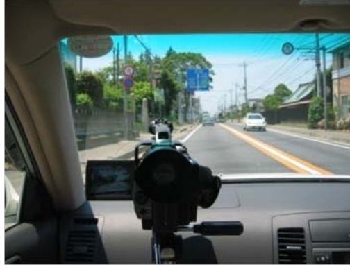
Figure 1.3: The video camera is mounted on a tripod firmly fixed at the front seat of a car.
