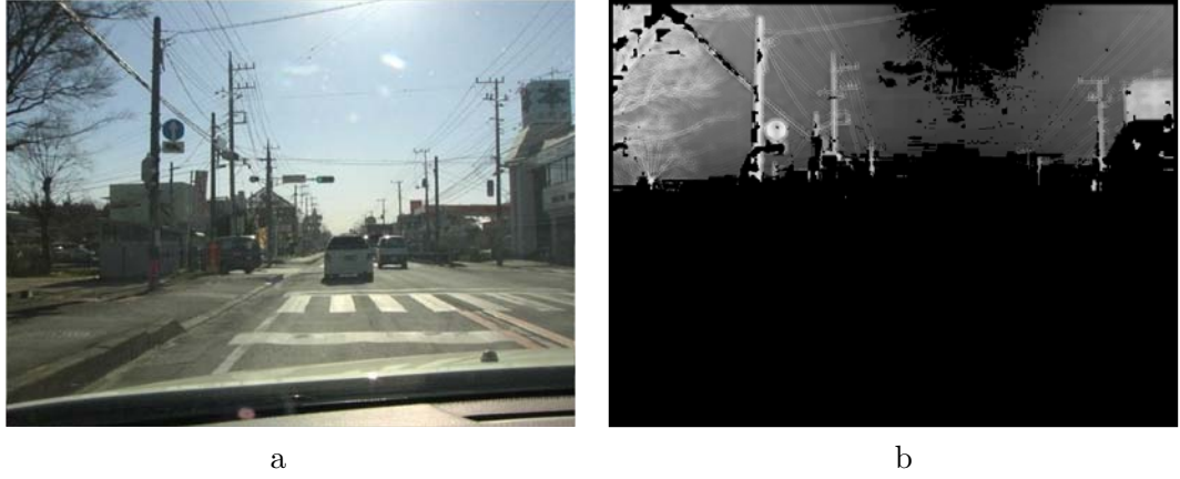
Figure 5.2: Example of an object which gives high response after applying opponent color filters although it is not a blue object. a: The original image. b: The output of opponent color filters.
