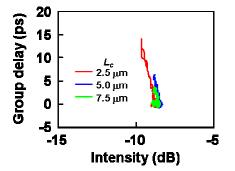
Fig. 10. GD-intensity plot of single peak nearest to 1550 nm in the spectra in Fig. 7.
