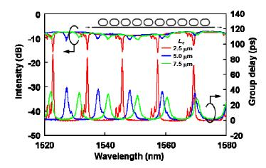
Fig. 11. Transmission spectra in intensity and GD of 10 cascaded RRs with  $R = 7.2 \ \mu\text{m}$  and  $L_c = 2.5, 5.0, \text{ and } 7.5 \ \mu\text{m}$ .
