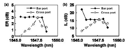
Fig. 16. Dependence of (a) ER and (b) IL on input wavelength in 10-Gb/s modulation experiments. Phase balance between the two arms was adjusted to obtain a constant ER from the bar port.
