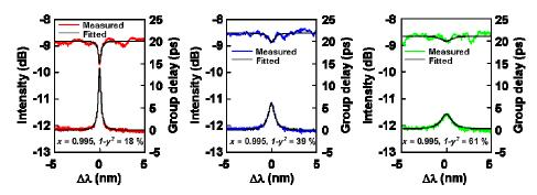
Fig. 8. Single peaks nearest to 1550 nm in intensity and GD spectra in Fig. 7. Measured curves are fitted by analytical formula of spectra for intensity and group delay derived from the Eq. (1), with the parameters of x and y. The values of x and y  $(1-y^2)$  used in the fittings are indicated in each graph. (a)  $L_c = 2.5 \,\mu\text{m}$ . (b)  $L_c = 5.0 \,\mu\text{m}$ . (c)  $L_c = 7.5 \,\mu\text{m}$ .
