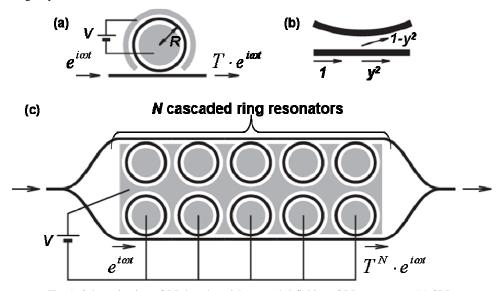
Fig. 1. Schematic view of RR-based modulators and definition of RR parameters. (a) SRR-SSM. (b) Coupling between ring and bus waveguide as a part of RRs.  $y^2$  and  $1 - y^2$  indicate the fraction of the power transmitted to the bus and the ring waveguide, respectively. (c) CRR-MZM.
