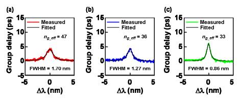
Fig. 5. Single peaks nearest to 1550 nm in GD spectra in Fig. 4. Measured curves are fitted by a Lorentzian function. (a)  $R = 2.5 \mu m$ . (b)  $R = 4.0 \mu m$ . (c)  $R = 7.2 \mu m$ .
