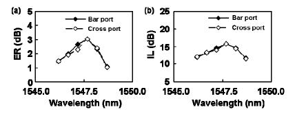
Fig. 15. Dependence of (a) ER and (b) IL on input wavelength in 10-Gb/s modulation experiments. Phase balance between the two arms was adjusted to obtain the same ER at the bar and cross ports.
