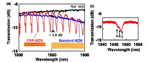
Fig. 13. (a) Measured transmission spectra of reference single passive waveguide (black), standard MZM (blue), and CRR-MZM (red). The photographs inside graph show device parts of test chip. (b) Close-up of single dip in the spectrum of the CRR-MZM. Arrows indicate wavelengths at which 10-Gb/s eye diagrams shown in Fig. 17 were measured.
