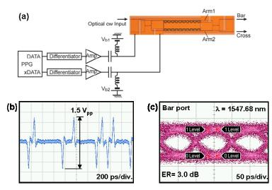
Fig. 14. 10-Gb/s large-signal modulation experiment using fabricated CRR-MZM. (a) Experimental setup. (b) Driving voltage waveform. (c) Eye diagram of optical output.
