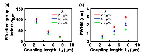
Fig. 9. Summary of GD characteristics of RRs with different values of *R* and  $L_c$  derived from single peak of GD nearest to 1550 nm in the spectra. Two samples were measured and analyzed for each combination of *R* and  $L_c$ . (a) Effective group index ( $n_{g,eff}$ ) and (b) FWHM.
