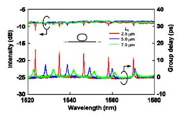
Fig. 7. Transmission spectra in intensity and GD of single RR with  $R = 7.2 \ \mu\text{m}$  and  $L_c = 2.5$ , 5.0, and 7.5  $\mu\text{m}$ .
