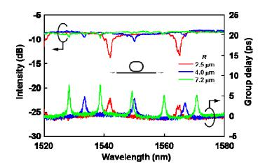
Fig. 4. Transmission spectra in intensity and GD of single RR with  $L_c = 5.0 \ \mu\text{m}$  and R = 2.5, 4.0, and 7.2  $\mu\text{m}$ .
