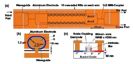
Fig. 12. Fabricated CRR-MZM. (a) Microscope photograph of top view. (b) Schematic view of one of cascaded RR in (a). (c) Schematic of cross section of dotted line in (b).
