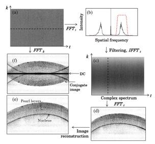
Fig. 5. (Color online) Flow diagram of full range image reconstruction process: (a) 2D spectral interferogram, (b) result of FFT of spectral interferogram in the lateral direction (dotted red curve indicates spatial frequency filter), (c) complex spectrum obtained after filtering and inverse FFT of (b), (d) full range image after FFT of complex spectrum in the optical wavenumber domain, (e) reconstructed full range image considering fiber motion, and (f) standard overlapping SD-OCT image.
