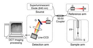
Fig. 1. (Color online) Schematic of a full range SD-OCT system based on a fiber-optic probe. C, collimator lens; M, mirror; L, lens; G, grating; FP, fiber-optic probe; S, sample.
