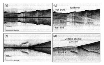
Fig. 6. Full range SD-OCT images of biological samples: (a) standard OCT image and (b) full range image of human fingernail near the nail fold region; (c) standard OCT image and (d) full range image of a human tooth near the dentino-enamel junction.
