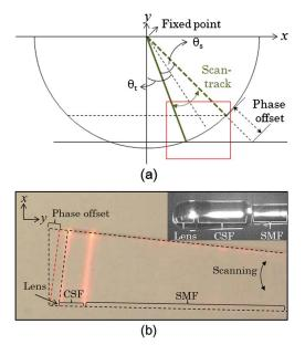
Fig. 3. (Color online) (a) Schematic diagram and (b) photograph of fiber end, illustrating the concept of phase offset in a fiber-based scanner.  $\theta_s$ , scan angle;  $\theta_t$ , tilt angle.
