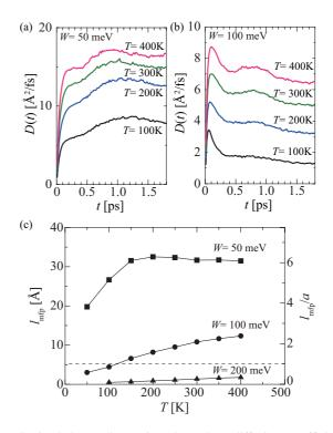
FIG. 6. (Color online) Time-dependent diffusion coefficients D(t) for temperatures from 100 to 400 K in the presence of static disorders with (a) W = 50 and (b) 100 meV. (c) Mean free path  $l_{\rm mfp}$  as a function of temperature T for W = 50, 100, and 200 meV, respectively. The ratios of  $l_{\rm mfp}$  to a are also shown in the right axis.
