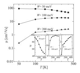
FIG. 5. Logarithmic plot of the carrier mobility  $\mu$  as a function of temperature *T* for the static disorders of W = 50, 100, and 200 meV, respectively. As *W* increases, the *T* dependence of  $\mu$  at around room temperature changes from the nearly power-law dependence to the thermally activated behavior. (Inset) Normal linear plots of  $\mu$  vs *T* characteristics for the static disorders of W = 50 (left), 100 (center), and 200 meV (right).
