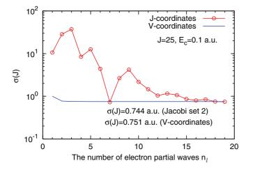
FIG. 3. (Color online) Partial protonium-formation cross sections obtained in the Jacobi coordinates (solid curve with open circles) and V coordinates (solid curve) as a function of the number of electron partial waves.
