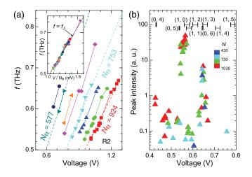
FIG. 4 (color online). Emission frequencies and intensities from R2. (a) Plots of f(V) for 8 branches in the R2 IVCs. Dashed lines: Fits to  $f = f_J = (2e/h)V/N_{\text{fit}}$ . Inset: Plot of  $f(V/N_{\text{fit}})$  for all R2 data. Dotted line:  $f = f_J$ . (b) Peak intensity on a logarithmic scale versus f for R2. Calculated  $f_{m,p}^c$  ranges are given at the top.  $N_{\rm fit}$  values are color-coded.
