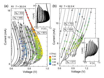
FIG. 2 (color online). Emission from IVC points at the colorcoded frequencies was observed at the filled diamonds. No radiation was detected at the open diamonds. Arrows indicate the numbers  $N_{\rm fit}$  of resistive junctions from fits to the Josephson relation. (a) *R*1. (b) *R*2. Insets: Full IVCs.
