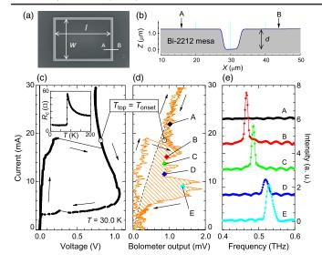
FIG. 1 (color online). *R*1 structure, *c*-axis resistivity, outermost-branch IVC, emission output, and frequency spectra. (a) Scanning ion microscope image. (b) Atomic force microscope image along *A*-*B* in (a). (c) Outer-branch IVC. Inset:  $R_c(T)$ . (d) Plot of  $I(V_{out})$  corresponding to (c). Open circles:  $T_{top} = T_{onset} = 84.4$  K. (e) Spectral intensities from points *A*-*E* in (d).
