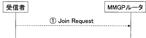
図4 非トークンメンバの加入 (MMGP Join) 手続き Fig. 4 Join procedure for the non-token member (MMGP Join).
