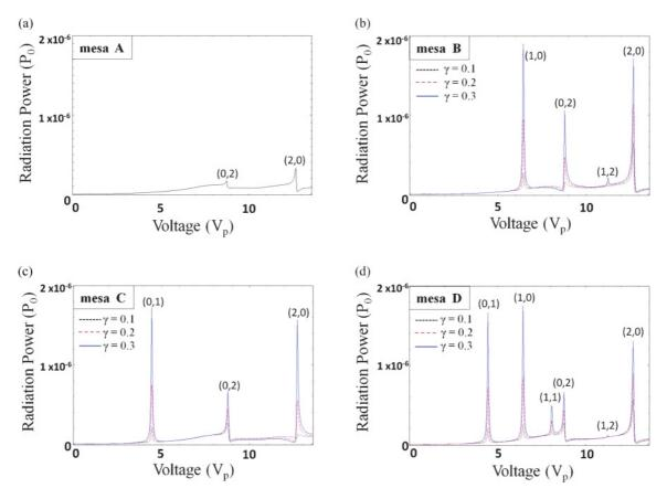
FIG. 3. (Color online) (a) The *P*-*V* curve of the homogeneous mesa. (b)–(d) The *P*-*V* curves of the inhomogeneous mesas with hot spots. The black (dotted), red (broken) and blue (solid) lines indicate the curves for  $\gamma = 0.1$ ,  $\gamma = 0.2$ , and  $\gamma = 0.3$  respectively.
