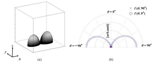
FIG. 8. (Color online) (a) The three-dimensional plots of  $I(\theta, \phi)$  at  $V = 12.7V_p$ . (b) The polar plots of  $I(\theta, 0^\circ)$  in the x-z plane and  $I(\theta, 90^\circ)$  in the y-z plane at  $V = 12.7V_p$ .
