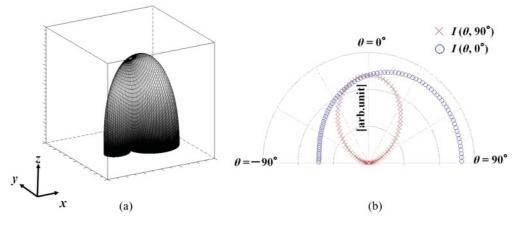
FIG. 7. (Color online) (a) The three-dimensional plots of  $I(\theta, \phi)$  at  $V = 6.44V_p$ . (b) The polar plots of  $I(\theta, 0^\circ)$  in the *x*-*z* plane and  $I(\theta, 90^\circ)$  in the *y*-*z* plane at  $V = 6.44V_p$ .
