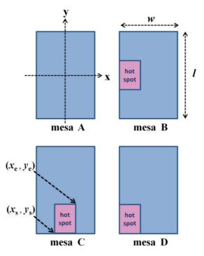
FIG. 2. (Color online) Schematic figures of the positions of the hot spots in the four different mesas.
