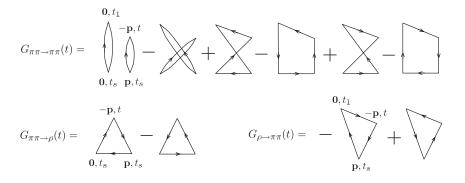
FIG. 2. Quark contractions of  $\pi\pi \to \pi\pi$ ,  $\pi\pi \to \rho$  and  $\rho \to \pi\pi$  components of the matrix of the time correlation function G(t). The time runs upward in the diagrams. The vertices refer to the pion or the  $\rho$  meson operator with the momentum at the time slice specified in the diagrams. The momentum **p** takes  $\mathbf{p} = (2\pi/L)(0, 0, 1)$  for the  $\mathbf{A}_2^-$  and  $\mathbf{p} = (2\pi/L)(1, 1, 0)$  for the  $\mathbf{B}_1^-$  representation.
