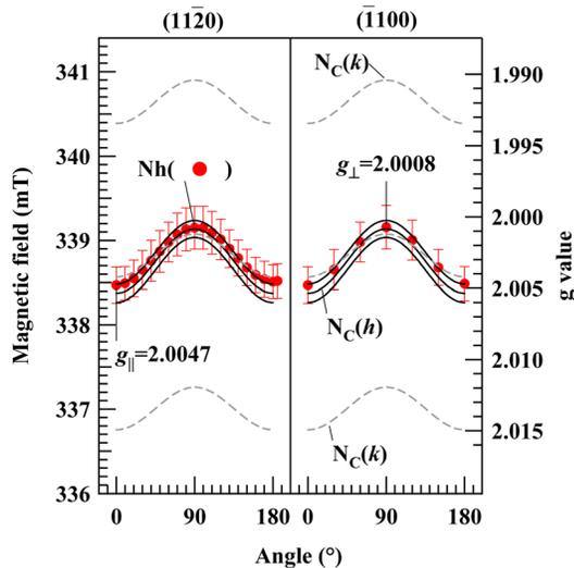
FIG. 3. (Color online) Angular maps of the Nh center (circles) and two nitrogen shallow donors,  $N_C(h)$  (solid lines) and  $N_C(k)$  (dashed lines). Error bars of Nh represent its peak-to-peak signal widths. Two angular maps were measured with respect to the  $\mathbf{B}$  rotation in the  $(11\bar{2}0)$  and  $(\bar{1}100)$  planes, where  $0^\circ$  angle represents that  $\mathbf{B} \parallel$  [0001].
