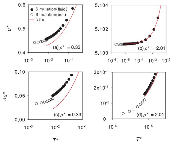
FIG. 7. The temperature dependence of  $u$  and  $\Delta u$  at  $\rho^* = 0.33$  ((a) and (c)) and  $\rho^* = 2.01$  ((b) and (d)). Filled and open circles represent the simulation results for the fluid and crystalline (bcc) phase, respectively. Solid lines are the RPA results for the fluid phase.
