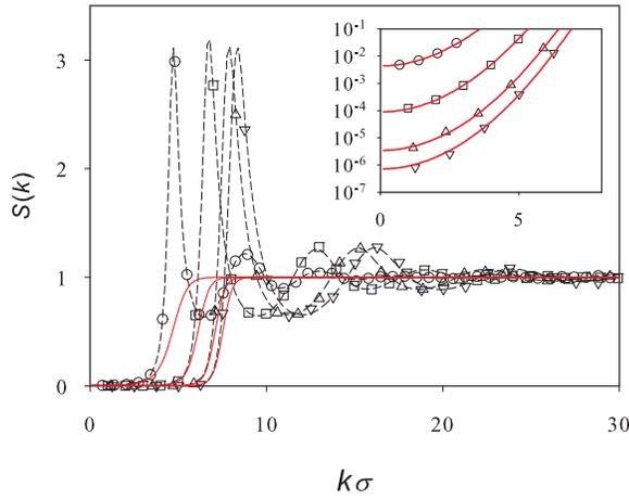
FIG. 5. The static structure factors in the fluid phase at the freezing temperatures for  $\rho^* = 0.33$  ( $\circ$ ), 1.00 ( $\square$ ), 1.65 ( $\triangle$ ), and 2.01 ( $\nabla$ ). The dotted lines are the results obtained by the Fourier transformation of  $g(r)$ . The solid lines are the results of RPA (see Sec. IV). The inset is the semi-log plot of the main figure for  $S(k) \leq 10^{-1}$  at low  $k$ 's.
