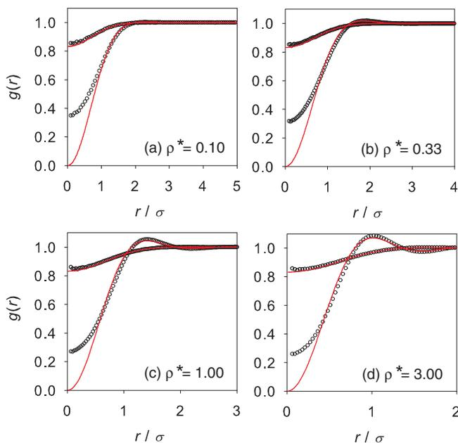
FIG. 6. The radial distribution function in the high temperature regime for (a)  $\rho^* = 0.10$ , (b) 0.33, (c) 1.00, and (d) 3.00. Circles and lines are simulation and RPA results, respectively. Two results in each panel correspond to the results at the threshold temperature ( $T^* = 0.823, 0.535, 0.159$ , and  $0.689 \times 10^{-2}$ ) and higher temperature at which  $g_{RPA}(r = 0) = 0.83$  ( $T^* = 5.76, 5.35, 4.30$ , and 2.29).
