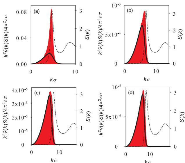
FIG. 9. The integrand of Eq. (9) (shaded areas), the integrand where  $S(k)$  is replaced with  $S_{RPA}(k)$  (solid lines) and  $S(k)$  (broken lines) for (a)  $T^* = 7.9 \times 10^{-3}$  and  $\rho^* = 0.33$ , (b)  $T^* = 5.0 \times 10^{-4}$  and  $\rho^* = 1.00$ , (c)  $T^* = 3.2 \times 10^{-5}$  and  $\rho^* = 1.65$  and (d)  $T^* = 7.9 \times 10^{-6}$  and  $\rho^* = 2.01$ .
