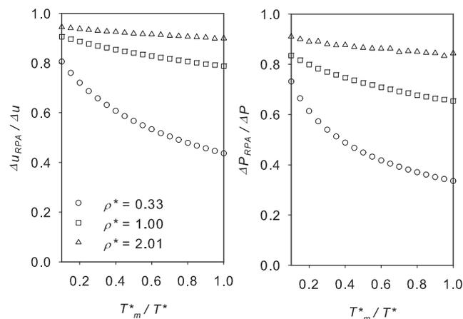
FIG. 8. Temperature dependence of the ratio of RPA to simulation values of the fluctuation part of the potential energy (left) and the pressure (right) for  $\rho^* = 0.33$  ( $\circ$ ), 1.00 ( $\square$ ), and 2.01 ( $\triangle$ ). The range of temperatures in these figures is much lower than the corresponding  $T_{th}$ . ( $T_m^*/T_{th}^*$  are  $1.48 \times 10^{-2}$ ,  $3.14 \times 10^{-3}$ , and  $2.55 \times 10^{-4}$  for  $\rho^* = 0.33, 1.00$ , and 2.01, respectively).
