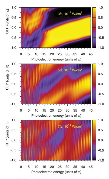
FIG. 5. (Color online) Asymmetry of ATI spectra of Ar at different laser pulse durations with a laser intensity of  $10^{14}$  W/cm<sup>2</sup>.
