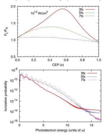
FIG. 2. (Color online) The ratios of total ionization probabilities to the left and right sides (upper panel) and the ATI spectra at  $\delta = 0$  (lower panel) of Ar in few-cycle laser pulses with a laser intensity of  $10^{13}$  W/cm<sup>2</sup>.
