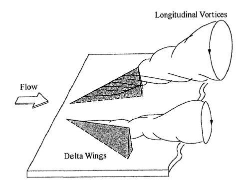
Figure 1.1 Longitudinal vortices generated by solid vortex generators.
