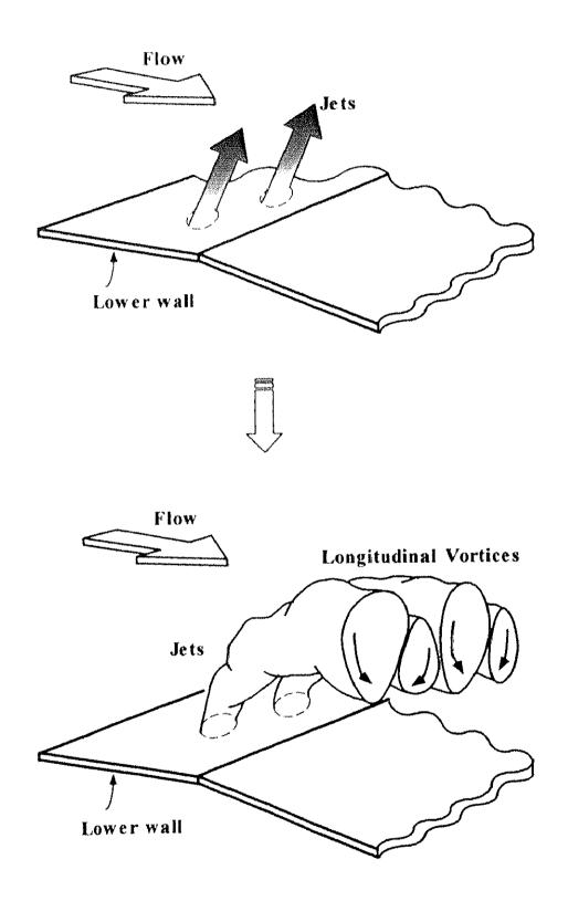
Figure 1.2 Longitudinal vortices due to jets issuing into freestream.
