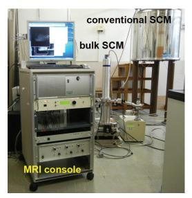
FIG. 1. (Color) The MR microscope developed in this study. The superconducting bulk magnet is seen in the center of the figure. The conventional superconducting NMR magnet used for energizing the bulk magnet is seen behind the bulk magnet.
