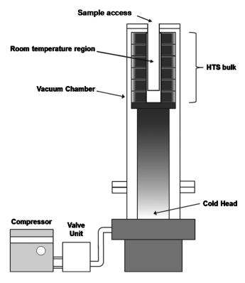
FIG. 2. Schematic of the HTS bulk magnet.
