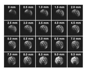
FIG. 4. 2D cross sections selected from a 3D image data set of a water capillary phantom. Numbers in the images are the vertical heights of the images. The voxel size is  $(100 \ \mu m)^3$ .
