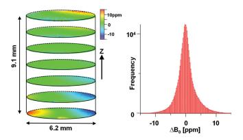
FIG. 3. (Color) Magnetic field distribution (left) and its histogram (right) measured in the central  $\phi$ 6.2mm $\times$ 9.1 mm region of the bulk magnet. Root mean square and peak-to-peak values of inhomogeneity were 3.1 ppm and 37 ppm, respectively.
