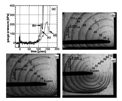
Fig. 8. Experimental results of Configuration C (shot6-8).  $C_2H_2+2.5O_2$  mixture, initial pressure of 70 kPa, initial temperature of  $282 \pm 1$  K. Pressure history is shown in (a).Wall distances  $z_w$  and  $x_w$  are 2.25 mm (b), 5.25 mm (c), 10.25 mm (d).
