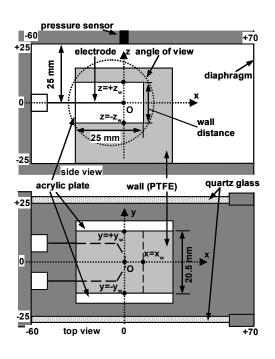
Fig. 9. Configuration D of the observation chamber. (single column - 215 words)
