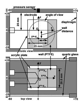
Fig. 7. Configuration C of the observation chamber. (single column - 215 words)
