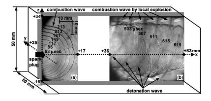
Fig. 3. Experimental results of Configuration A.  $C_2H_4+3O_2$  mixture, initial pressure of 60 kPa, initial temperature of 294±1 K, left - shot1 (32 msec/flame), right - shot2 (4 msec/flame). (double column - 283 words)
