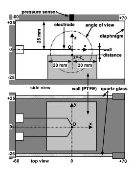
Fig. 5. Configuration B of the observation chamber. (single column - 215 words)
