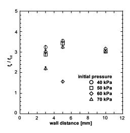
Fig. 11. Experimental result of Configuration D (shot9-20).  $C_2H_2+2.5O_2$  mixture, initial temperature of  $284 \pm 1$  K. Wall distance versus  $t_e/t_{c2}$ . (single column - 180 words)
