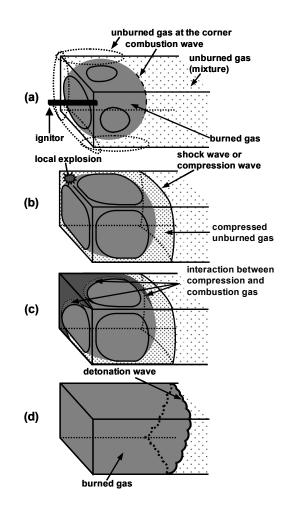
Fig. 1. Detonation initiation by local explosion near a closed end. (single column - 302 words)
