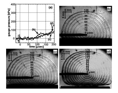
Fig. 6. Experimental results of Configuration B (shot3-5). $C_2H_2+2.5O_2$  mixture, initial pressure of 70 kPa, initial temperature of 283±0 K. Pressure history is shown in (a).Wall distances  $z_w$  are 2.25 mm (b), 5.25 mm (c), 10.25 mm (d).
