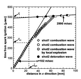
Fig. 4. Trajectories of combustion wave front and detonation wave. (single column - 167 words)
