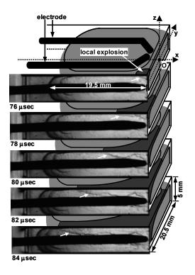
Fig. 10. Shot16, explosion in closed end.
