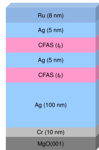
Fig. 4-15 Layer structure of the pseudo spin-valve.
