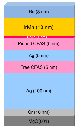
Fig. 4-12 Layer structure of the exchange biased spin-valve.
