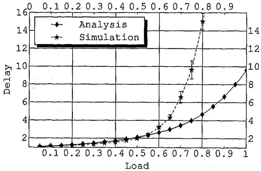
Figure 8: Average packet delay versus load ( $T = 100, M = 50$ ).
