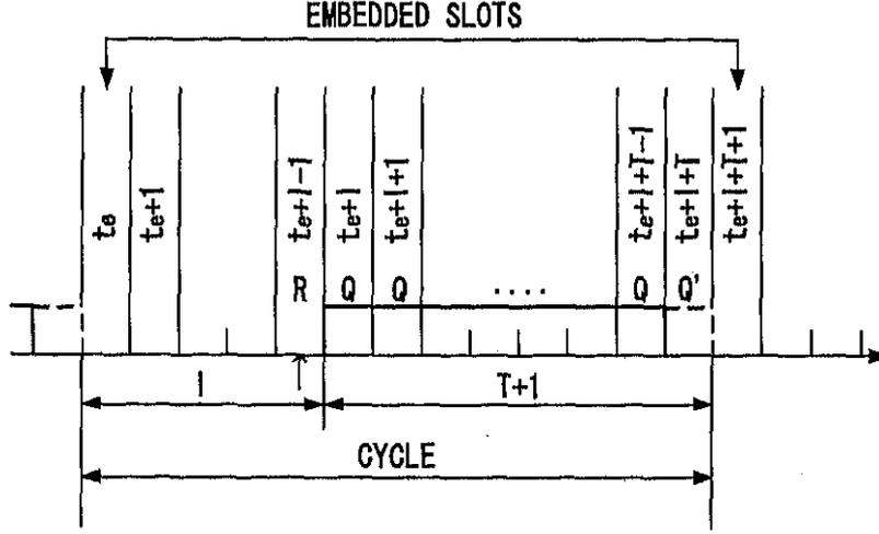
Figure 2: Imbedded slots in a model of CSMA/CA.
