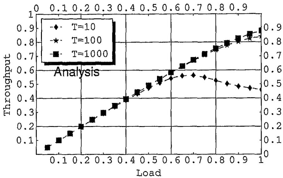
Figure 3: Throughput versus load by analysis ( $M = 50$ ).
