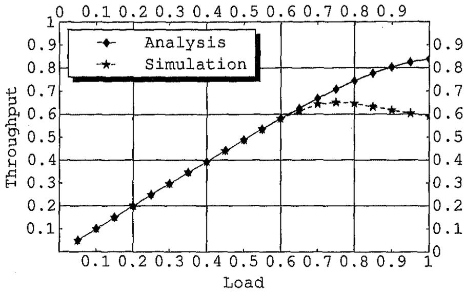
Figure 7: Throughput versus load ( $T = 100, M = 50$ ).
