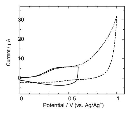
Figure 4. Cyclic voltammograms of poly(DFCz0) at a scan rate of 100 mV/s with a scan range up to 0.6 V (solid line) and a scan range up to 1.0 V (dashed line).
