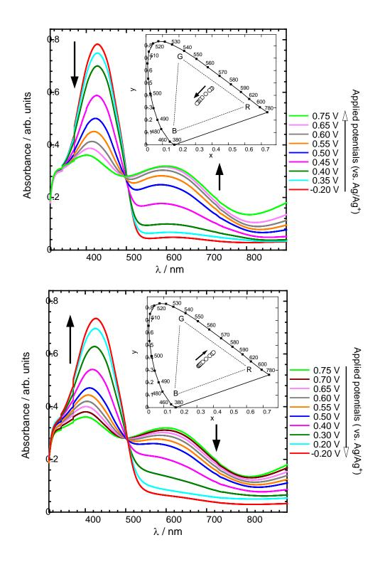
Figure 6. UV-vis absorption spectra of poly(DTCz4) at various applied potentials (vs.  $Ag/Ag^+$ ) (top; oxidation process, bottom; reduction process). Insets show CIE color coordinates of the polymer.
