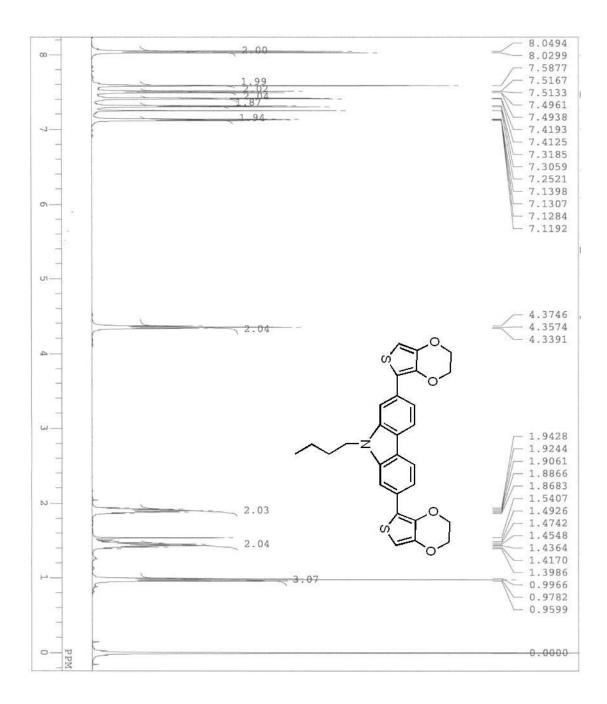
Figure S22. <sup>1</sup>H NMR spectrum of *N-butyl-2,7-di(2-(3,4-ethylenedioxythienyl))carbazole* (*DECz4*).
