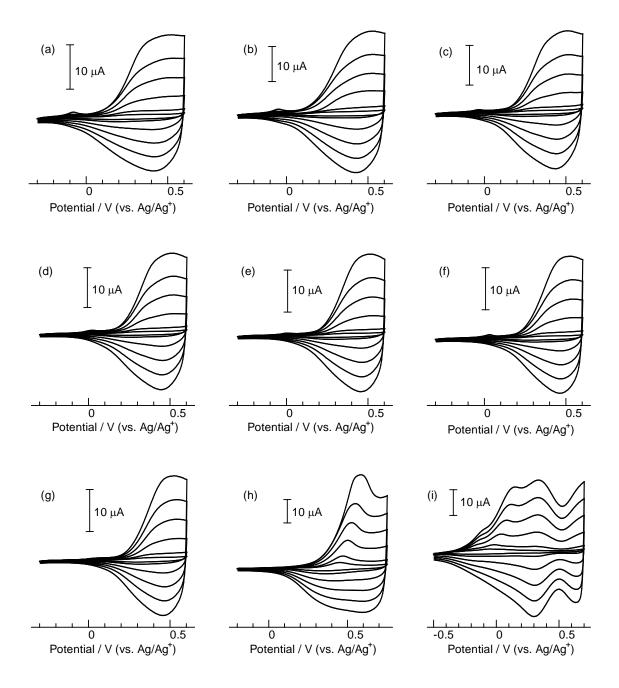
Figure 3. Cyclic voltammograms of the polymers deposited on a platinum disc electrode at various scan rates (10, 20, 40, 60, 80, and 100 mV/s) (vs. Ag/Ag<sup>+</sup>) ((a); DFCz0, (b); DFCz1, (c); DFCz2, (d); DFCz3, (e); DFCz4, (f); DFCz5, (g); DFCz6, (h); DTCz4, (i); DECz4).
