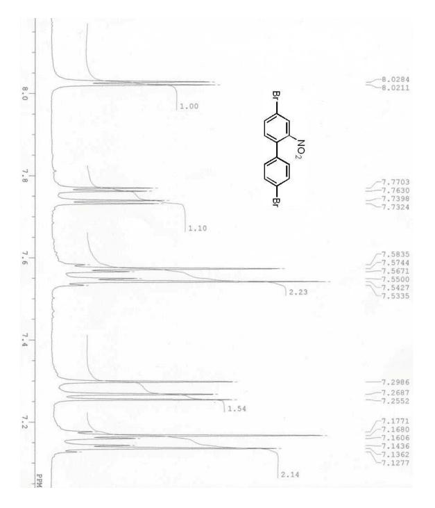
Figure S6. <sup>1</sup>H NMR spectrum of 4,4'-Dibromo-2-nitro-biphenyl (2).
