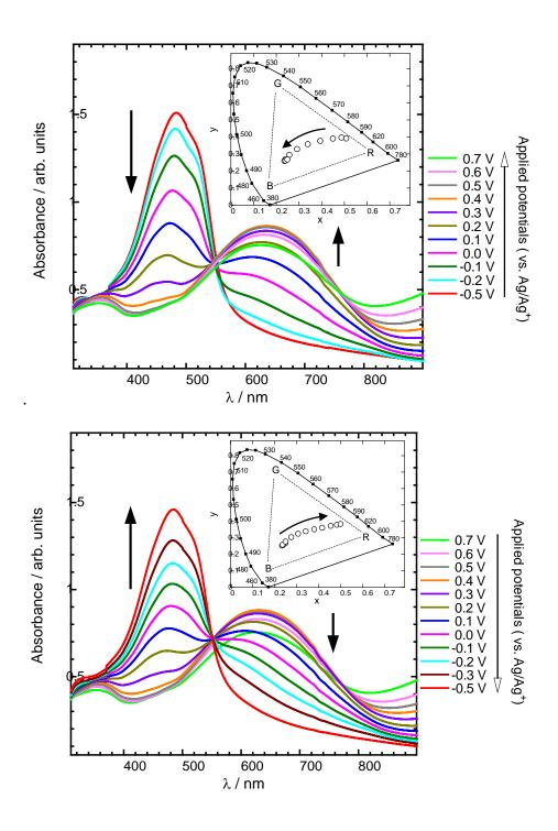
Figure 7. UV-vis absorption spectra of poly(DECz4) at various applied potentials (vs.  $Ag/Ag^+$ ) (top; oxidation process, bottom; reduction process). Insets show CIE color coordinates of the polymer.
