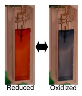
Figure 8. Photographs of the poly(**DECz4**) film in the reduced state (-0.5 V vs. Ag/Ag<sup>+</sup>) (left) and the oxidized state (0.7 V vs. Ag/Ag<sup>+</sup>) (right).
