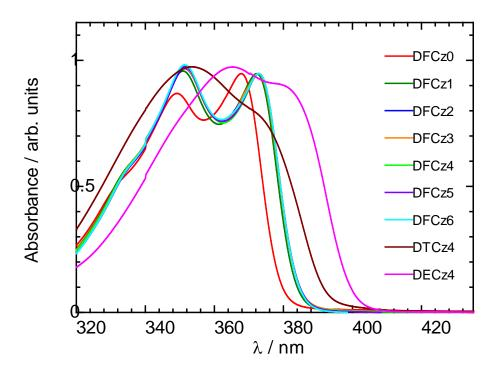
Figure 2. UV-vis absorption spectra of the monomers in chloroform solutions.
