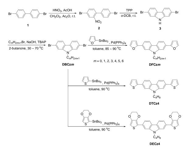
Scheme 1. Synthesis of four-rings type carbazole monomers. (AcOH; acetic acid, Ac<sub>2</sub>O; acetic anhydride, TPP; triphenyl phosphine, *o*-DCB; *o*-dichlorobenzene, SnBu<sub>3</sub>; tributylstannyl group, TBAP; tetrabutylammonium perchlorate)
