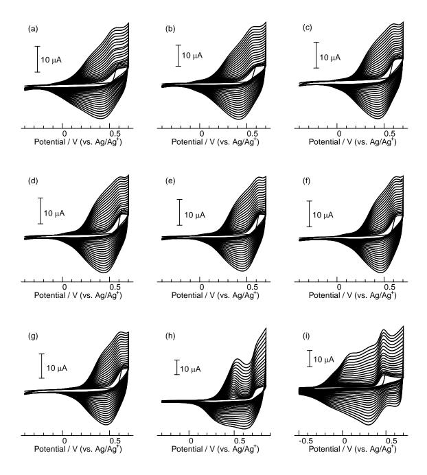
Figure 1. Electrochemical polymerization of the 2,7-heteroaromatic substituted carbazole monomers ((a); DFCz0, (b); DFCz1, (c); DFCz2, (d); DFCz3, (e); DFCz4, (f); DFCz5, (g); DFCz6, (h); DTCz4, (i); DECz4).
