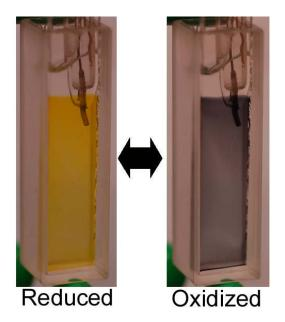
Figure S5. Photographs of the poly(**DTCz4**) film in the reduced state (-0.2 V vs. Ag/Ag<sup>+</sup>) (left) and the oxidized state (0.75 V vs. Ag/Ag<sup>+</sup>) (right).
