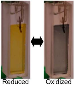
Figure S4. Photographs of the poly(**DFCz4**) film in the reduced state (-0.3 V vs. Ag/Ag<sup>+</sup>) (left) and the oxidized state (0.6 V vs. Ag/Ag<sup>+</sup>) (right).
