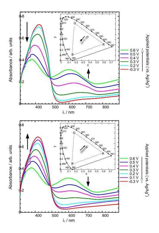
Figure 5. UV-vis absorption spectra of poly(DFCz4) at various applied potentials (vs.  $Ag/Ag^+$ ) (top; oxidation process, bottom; reduction process). Insets show CIE color coordinates of the polymers.
