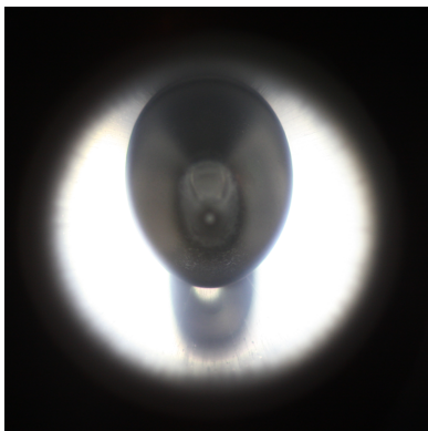
Fig. 2-4 Solid hydrogen by a pressure of 67 mbar. When hydrogen was solidified at low pressure (hydrogen supply pressure below 100 mbar), a large void was remained.
