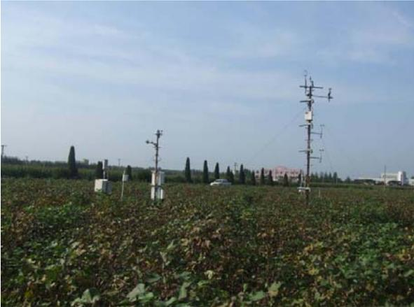
**Fig.5-10** The APEIS-Flux station in the cotton field.
