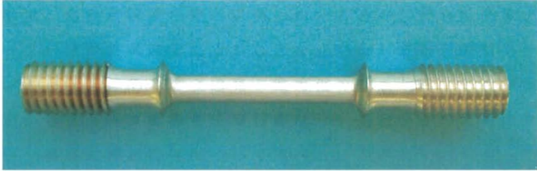
Fig. 1-9 A creep test specimen used in this study, prepared to JIS-Z2271 standard (length: 60mm, gauge length: 20mm, radius: 4mm).
