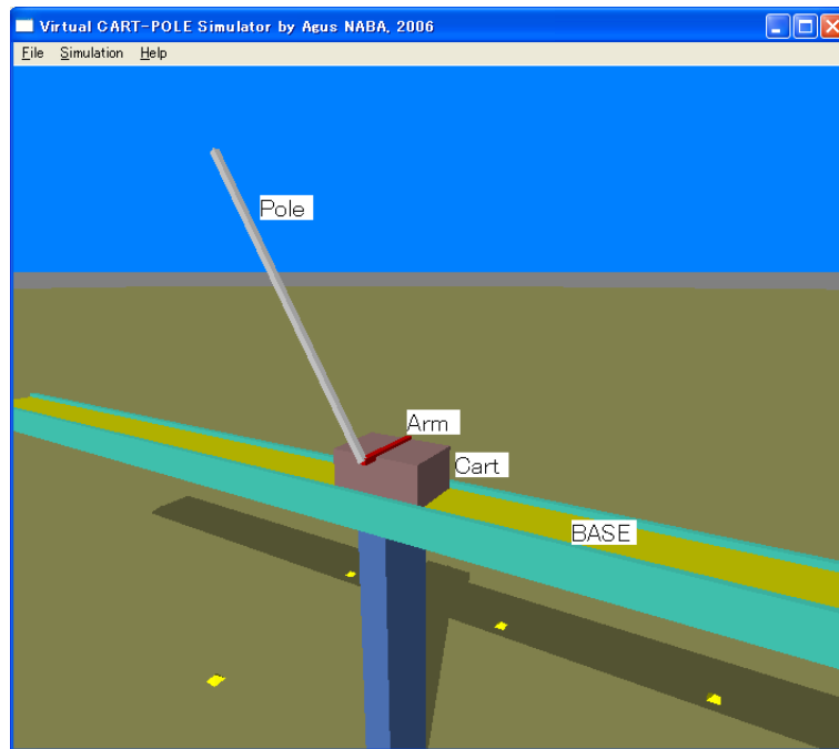
Figure 4.14: Virtual cart-pole plant
