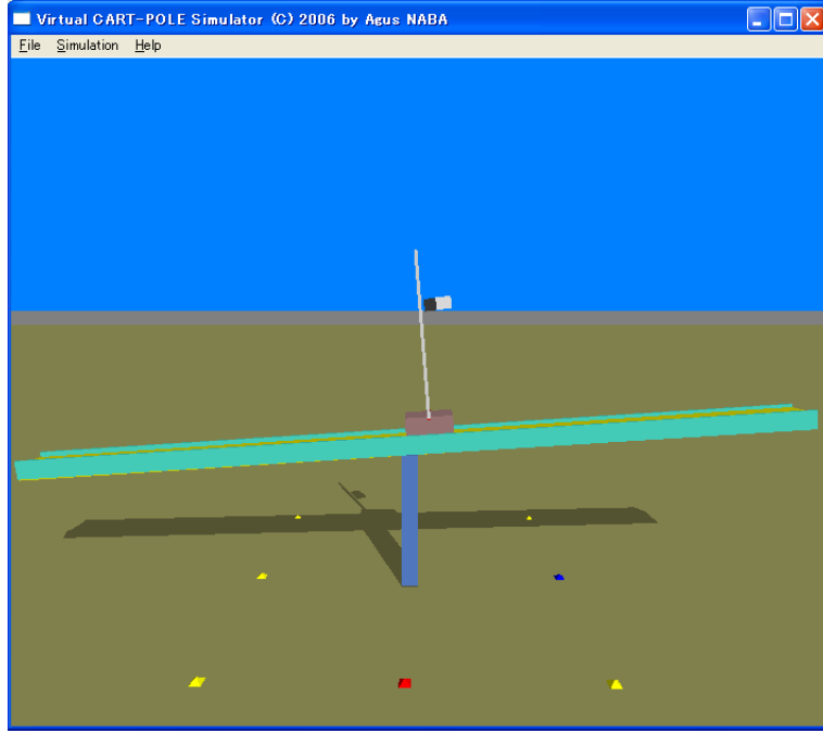
Figure 4.16: Control of ODE cart-pole plant subject to perturbations, i.e., the base is inclined and a box is thrown to the pole
