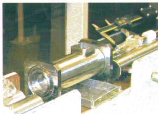
<<Chamber for mercury>>
