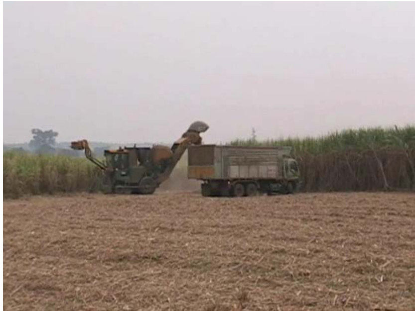
Figure C-1 Turning operation at a headland
