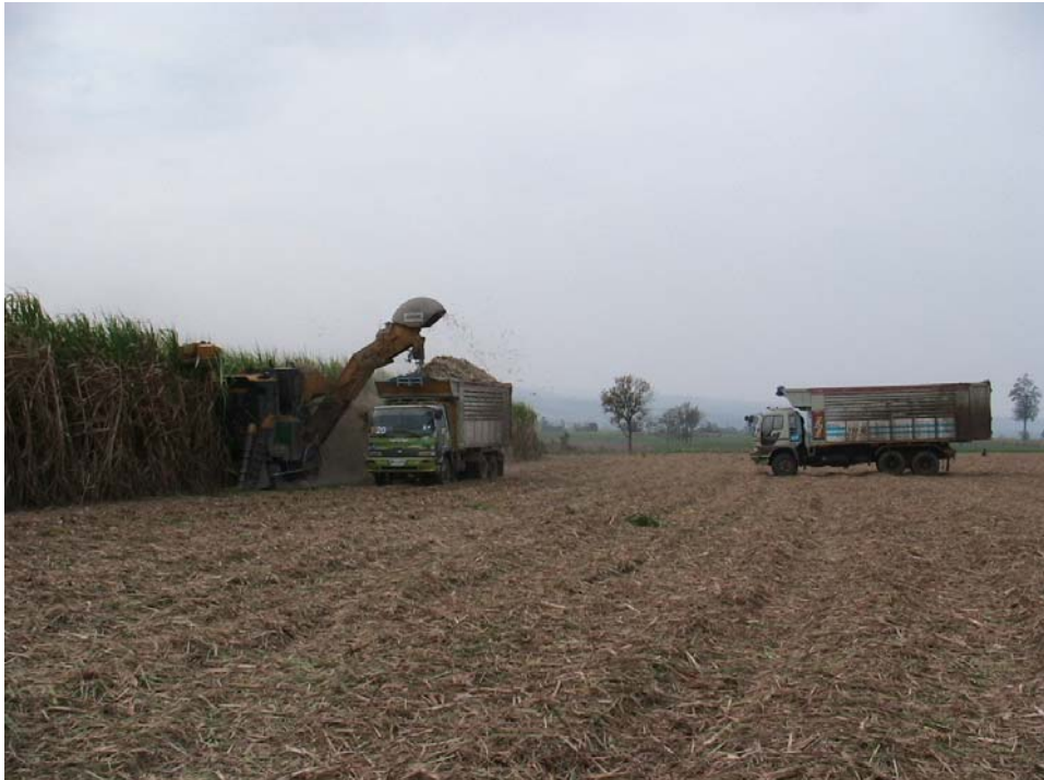
Figure 2.2 The chopper-type mechanical sugarcane harvester
