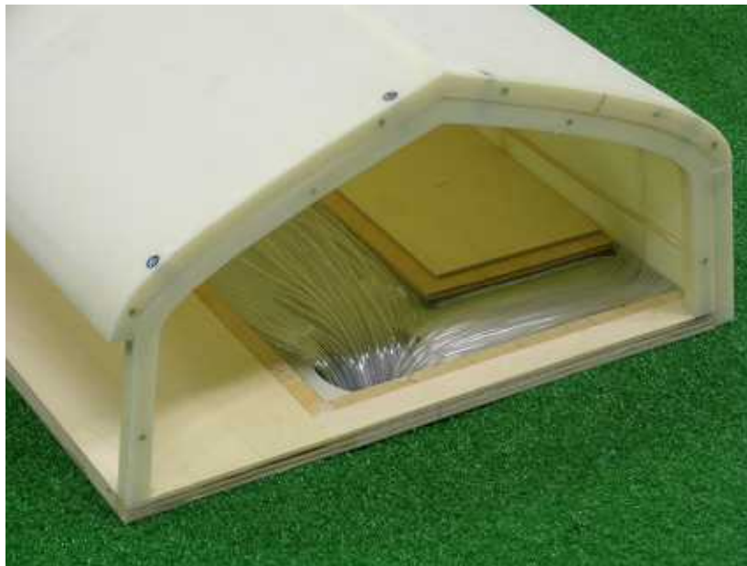
Fig. 4.5 Model consists of a sandwich structure for tubes connecting between pressure taps and electronic pressure scanning system.
