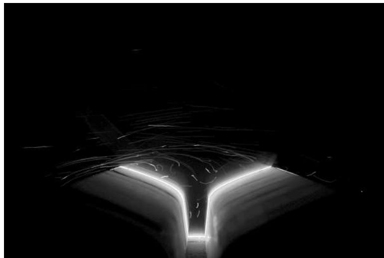
Fig. 5.11 Visualization of air flow using laser sheet and micro bubbles.
