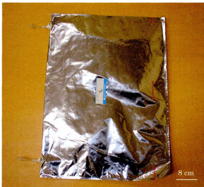
**Figure 3.5** Aluminum sampling gas bag CCK (20 L) used in the different experiments. The two outlets disposed two mini valves.
