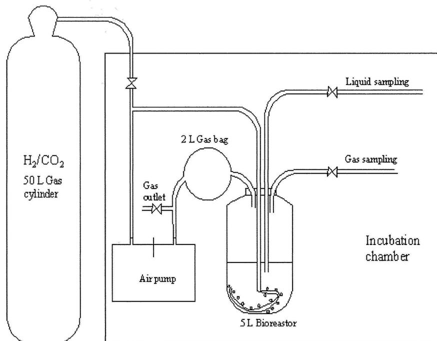
**Figure 3.1** Schematic diagram for hydrogenotrophic methanogens acclimation.
