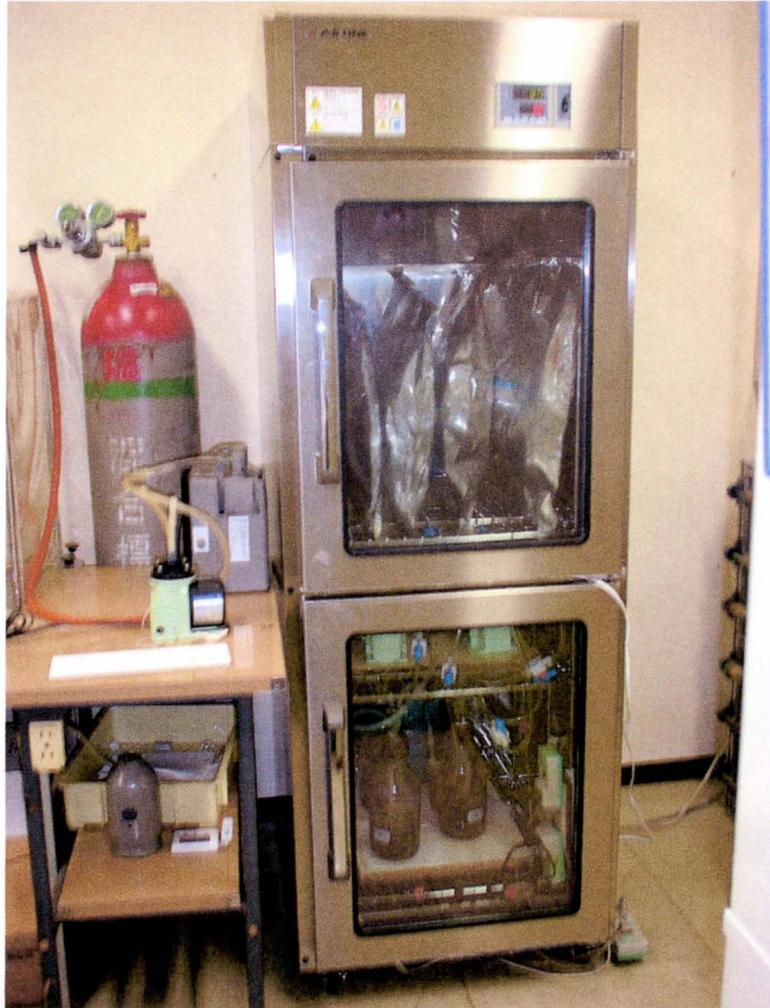
**Figure 4.1** Experimental incubation chamber with the four reactors systems
