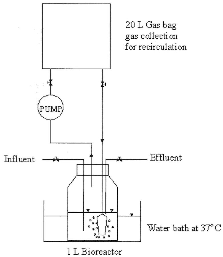
**Figure 3.4** Schematic diagram for experimental bioreactor.
