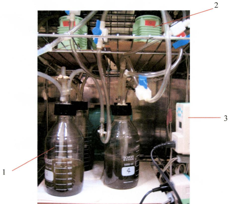
1 Chemostat reactor; 2 Airtight pump; 3 Timer for mixing duration control
