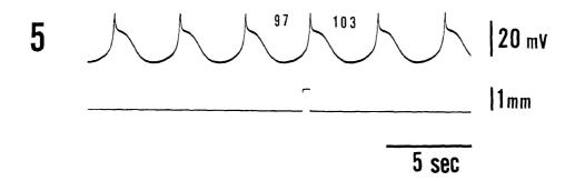
Fig. 13. Effect of a brief stretch on the electrical activity and on the beat interval. Records were taken intracellularly from the isolated ventricle. Upper trace; membrane potential, lower trace; monitor of stretch. The phases (%) where the stretch was applied are 12, 28, 45, 66 and 90 % in records 1-5, respectively. Interval change is shown by % relative to the preceding control interval (100 %).
