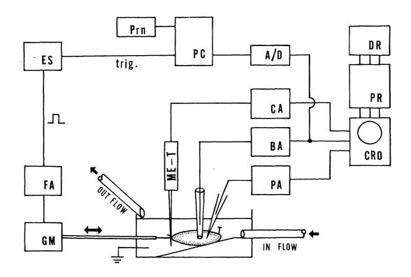
Fig. 12. Schematic representation of the experimental arrangement; ME-T, mechanoelectro-transducer; CA, carrier amplifier; BA, biological AC amplifier; PA, pre-amplifier; CRO, cathode ray oscilloscope; PR, pen-writing oscillograph; DR, magnetic data recorder; A/D, analogue to digital converter; PC, micro-computer; Prn, dot-impact printer; ES, electronic stimulator; FA, feed-back amplifier; GM, galvanometer.
