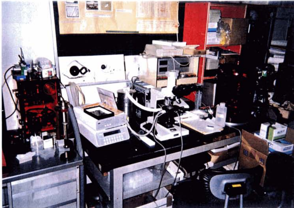
Figure 6. Diagram of the heating stage and appearance. The fluid inclusions were experimented by the heating and cooling stage of the Linkam THM-600 with the error of 5 °C.
