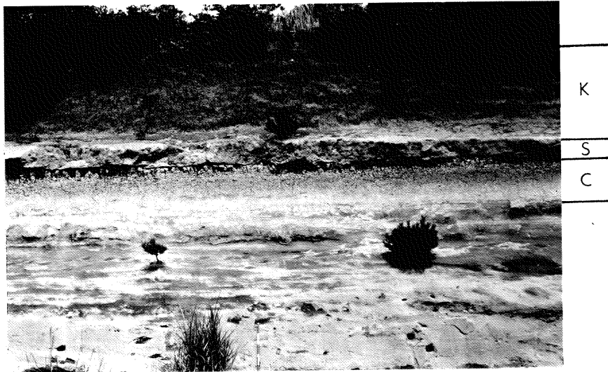
Photograph 4 Slope T3-SW viewed from the southwest. A measure at middle of bottom is 80 cm long. August 1981. K: Kanto Loam, S: Sandy bed, C: Clayey bed.
