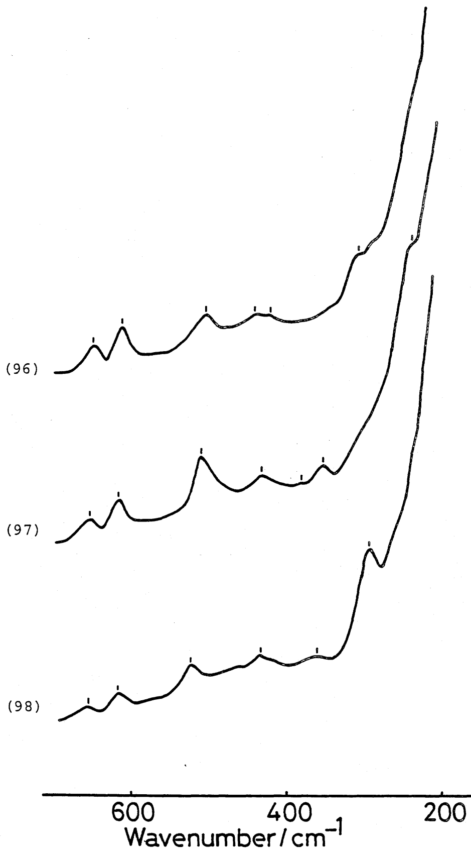
Figure 56. Raman spectra of three geometrical isomers of [\text{Co}(\text{L-smc})_2]^+ . Numbers in parentheses correspond to those in Table 16.
