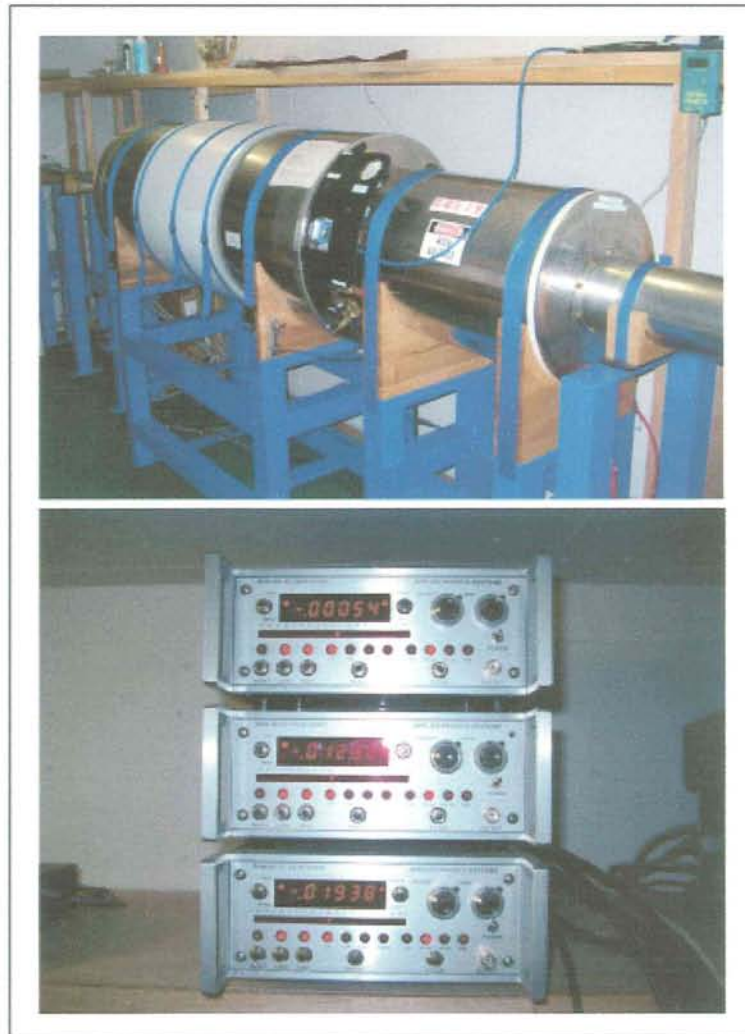
Photo 9. AFD Laboratory used for alternating field demagnetization analyses. Up: AFD demagnetizer unit model 2G-760, down: SQUID model 581DC.
