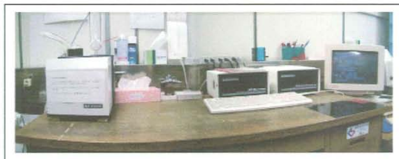
Photo 10. Laboratory of Magnetic Susceptibility used for AMS and thermomagnetic analyses. From left to right: KappaBridge pick-up unit model KLY-3, KappaBridge susceptibility meter model KLY-3S, Temperature control unit model CS-3 and computer control center.
