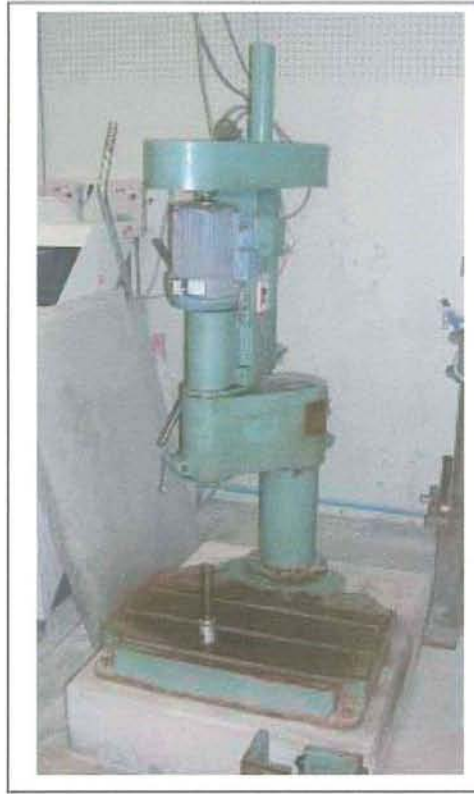
Photo 7. Driller machine at the University of Tsukuba used to prepare paleomagnetic cores.
