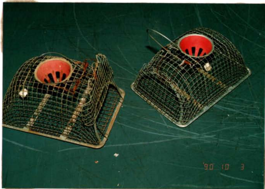
Fig.2-16 The trap for the rat made of wire mesh with a piece of cheese. (left: the entrance is open, right: the entrance is closed)
