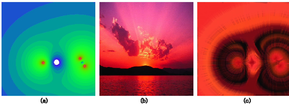
Figure 5-16. (a) image of vector field magnitude value (b) sunset image used as color palette (c) Color Stealing based LIC results
