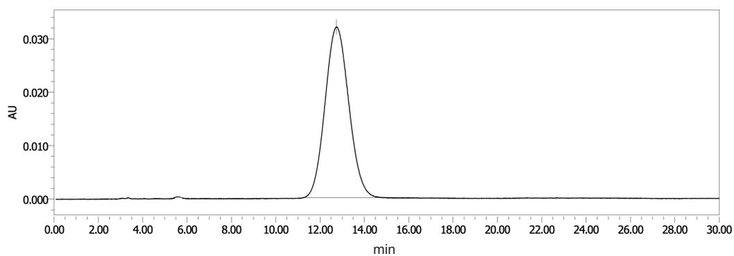
**Figure S15.** Chiral HPLC chromatogram of isolated **(-)-52a** with Chiralpak AD-H (Eluent: hexane/2-propanol = 1/1, Flow rate: 1 mL/min).
