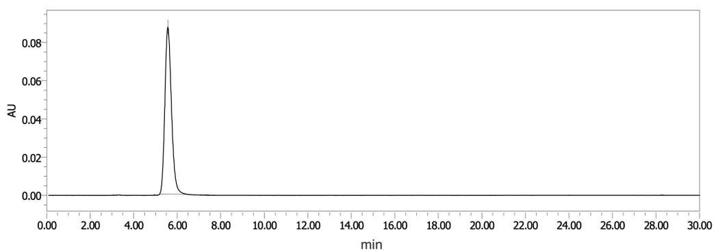
**Figure S14.** Chiral HPLC chromatogram of isolated **(+)-52a** with Chiralpak AD-H (Eluent: hexane/2-propanol = 1/1, Flow rate: 1 mL/min).
