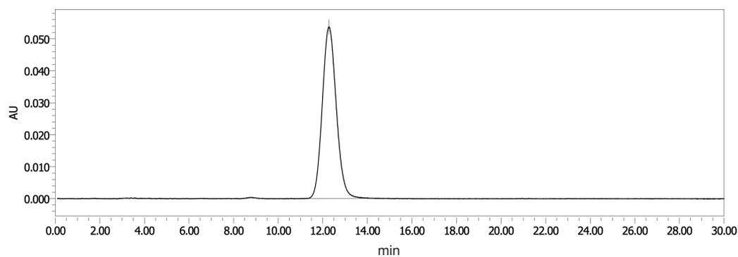
**Figure S18.** Chiral HPLC chromatogram of isolated (-)-**52d** with Chiralpak AD-H (Eluent: hexane/2-propanol = 3/2, Flow rate: 1 mL/min).
