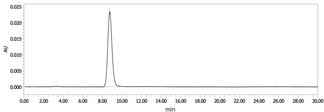
**Figure S17.** Chiral HPLC chromatogram of isolated (+)-**52d** with Chiralpak AD-H (Eluent: hexane/2-propanol = 3/2, Flow rate: 1 mL/min).
