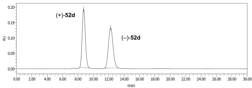
**Figure S16.** Chiral HPLC chromatogram of **52d** as racemic mixture with Chiralpak AD-H (Eluent: hexane/2-propanol = 3/2, Flow rate: 1 mL/min).
