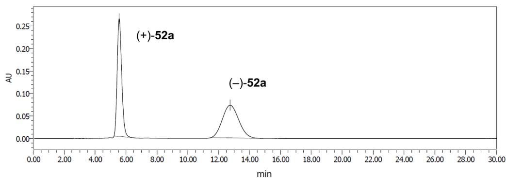
**Figure S13.** Chiral HPLC chromatogram of **52a** as racemic mixture with Chiralpak AD-H (Eluent: hexane/2-propanol = 1/1, Flow rate: 1 mL/min).
