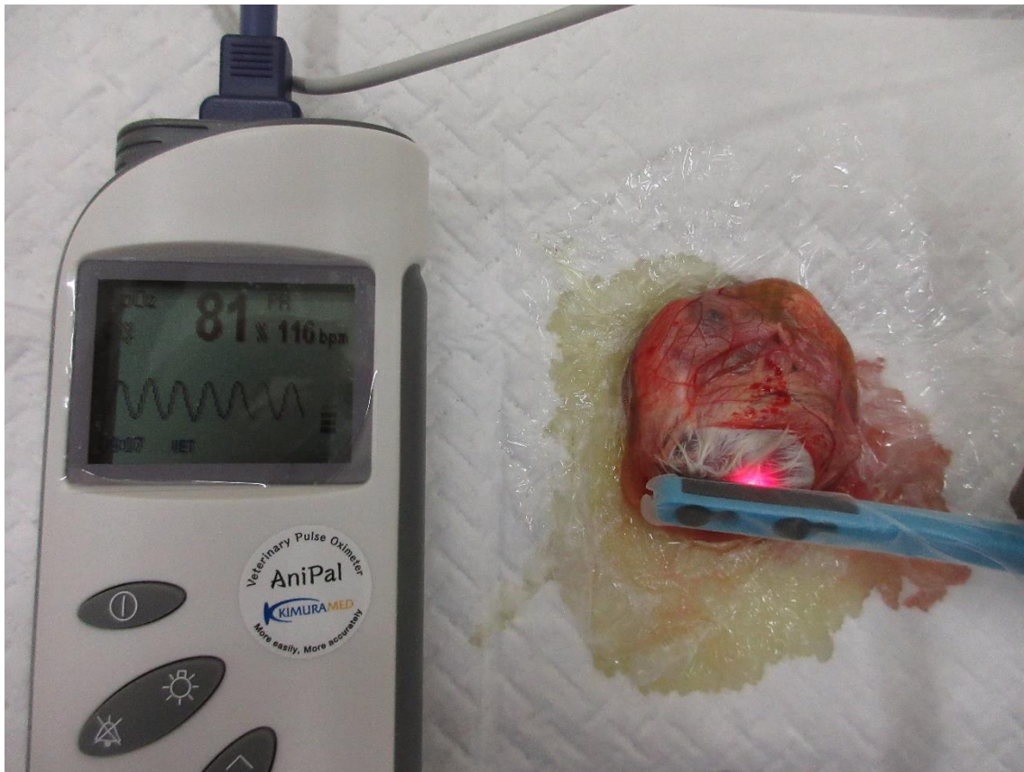
Figure 3-1. SpO 2 measurement of an embryo cultured in a cSLC using a pulse oximeter on day 19 of culture.
