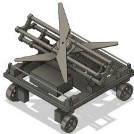
Figure 5-1 Computer-aided design of the proposed grass-cutting robot.
