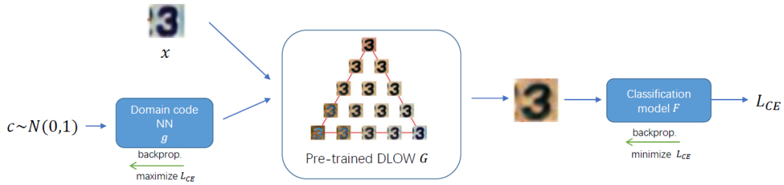
Figure 3.3: An overview of GADA with the domain-code NN. The domain-code NN takes Gaussian noise as input and outputs a valid domain code. The pretrained DLOW takes both image x and domain code as input and synthesizes an image with the style specified by the domain code. The classification model is trained with synthesized images. We optimize the domain code-NN to maximize the classification loss so that it can represent the worst-case distribution.
