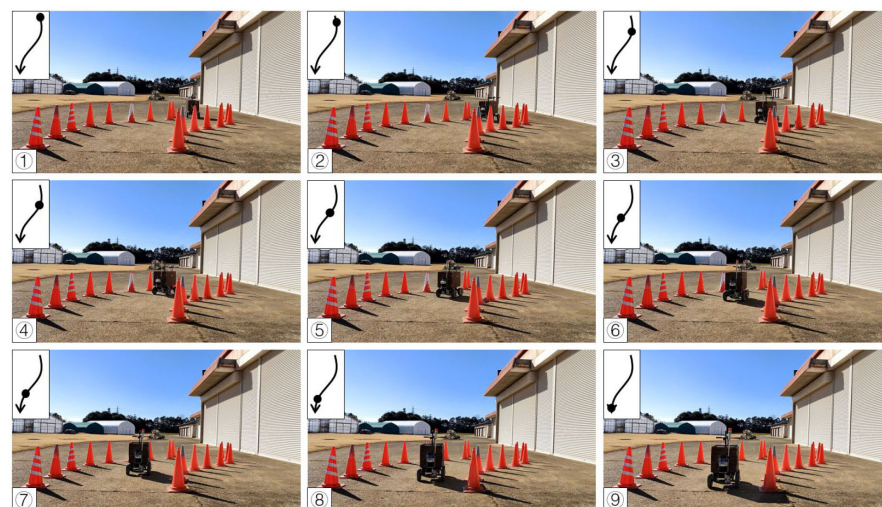
Figure 13. Curve path calibration on the concrete road (right turn). Subfigures (1–9) in order were the vehicle's movement path.
