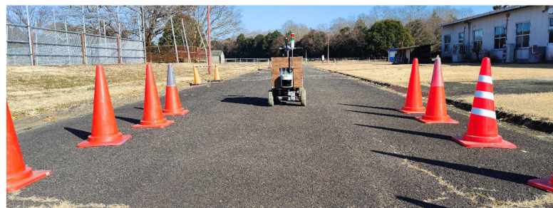
Figure 11. Calibration of the LiDAR sensor and the robot on the concrete road (cones were used instead of trees).
