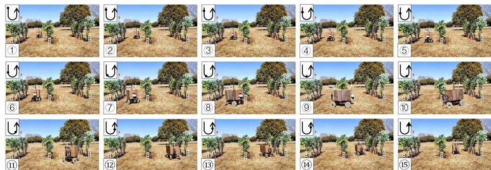
Figure 26. Images of vehicle operation in the facilitated artificial-tree-based orchard (left turn). Subfigures (1–15) in order were the vehicle’s movement path.
