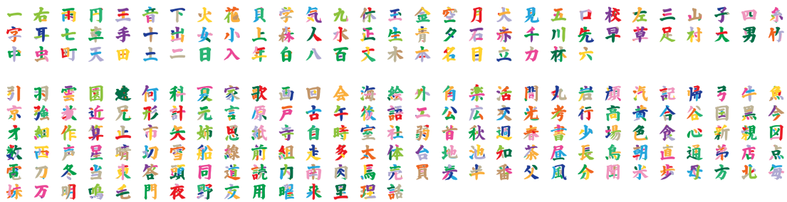
Figure 7.2: Stroke segmentation of HGHakushuGokubutoKaishota by moji-disassembler: From the looks of it, stroke segmentation is correctly achieved in about half of the strokes, but there are a few areas that are not segmented correctly. The strokes are jagged in places and have more of a brush stroke feel.
