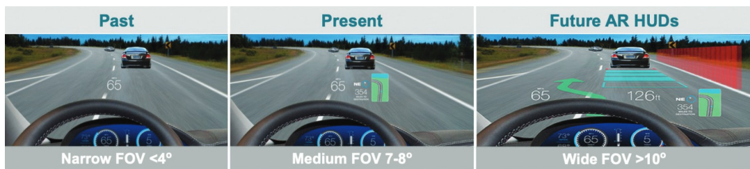
FIGURE 2.3: Future AR-HUDs will allow for a FOV of 10 degrees or more and overlay graphics directly onto the real world
