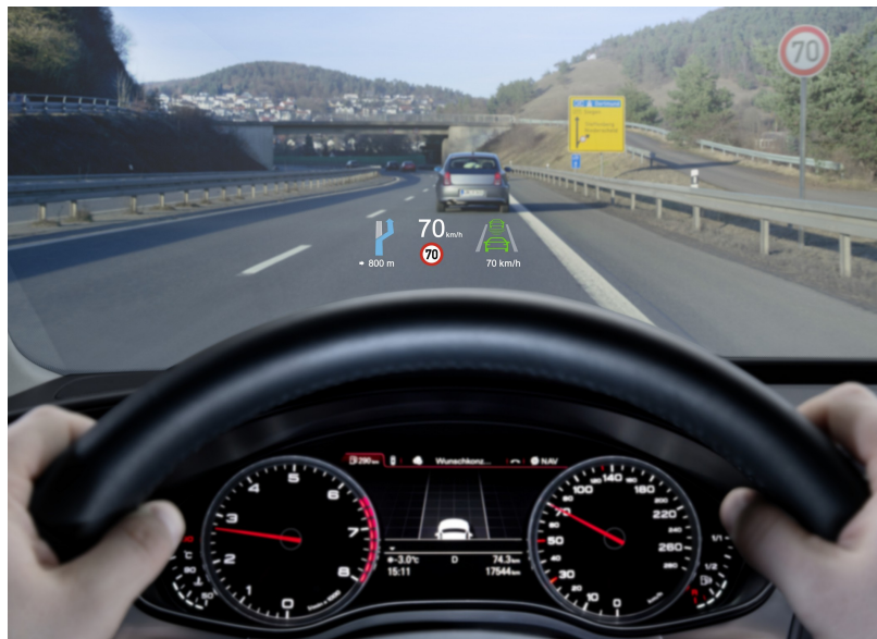
FIGURE 2.1: The second generation head-up display from Continental is also in series production in the Audi A6 and A7
