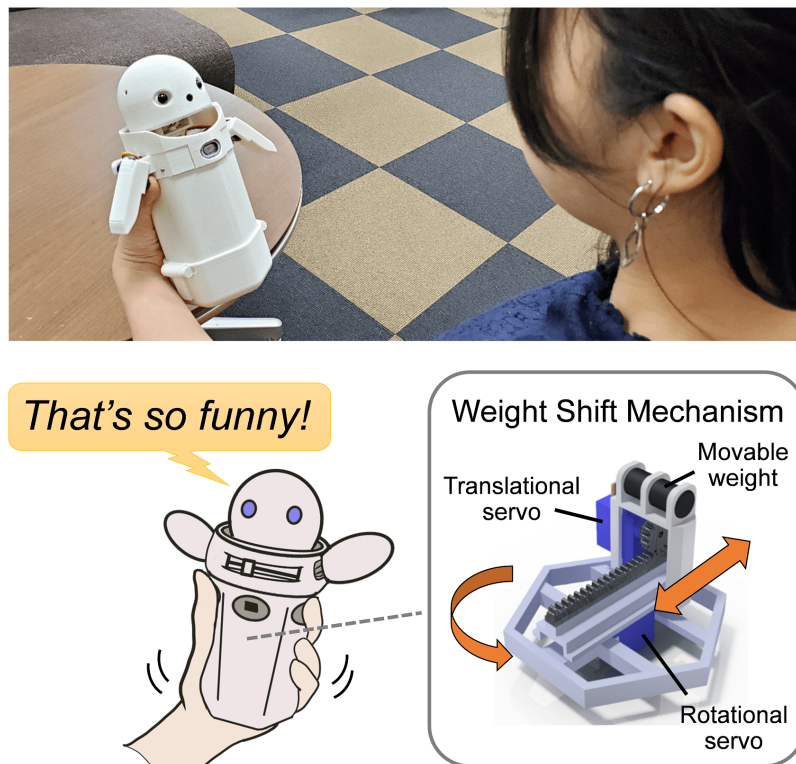
Fig. 7.1 The robotic gadget, named OMOY, developed in this study can exhibit various weight shifts to express emotions and intentions. A movable weight is implemented inside its body and is controlled by the translational and rotational mechanisms determined by four parameters (target position, trajectory, speed, and repetition). By exhibiting appropriate weight shifts together with gestures or speech dialogues, emotional and intentional messaging between users is expected to be enhanced.
