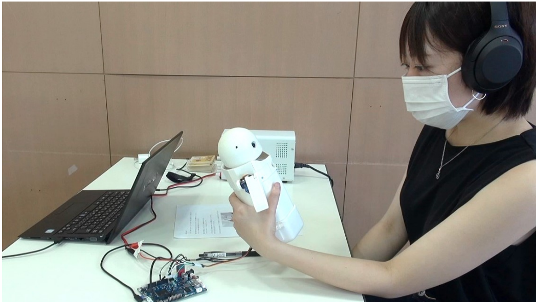
Fig. 8.3 The experiment was conducted at a booth constructed in a cafeteria in the University of Tsukuba. Each participant was asked to hold OMOY and tested one of its behaviors generated by speech and weight shifts. An experimenter took a seat in front of the participant.
