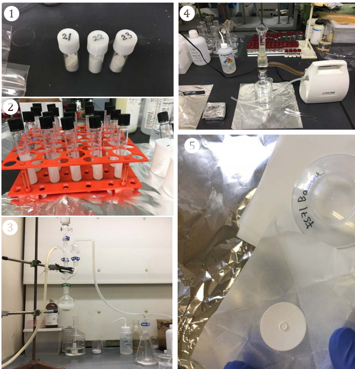
Figure 9. The photographs of the sample preparation for isotope measurements. 1) Cleaned and powdered samples, 2) Leaching with H_2O_2 , 3) Rinsing in deionized water under N_2 gas atmosphere, 4) Filtering for BaSO_4 residue, and 5) The ready residue of the BaSO_4 for measurement.
