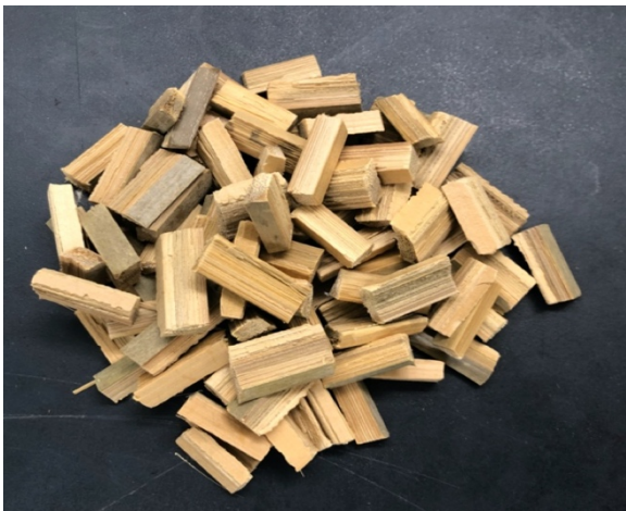
Dried bamboo was cut into chips with a size of 0.5 cm thickness * 1.0 cm width * 2.0 cm length
